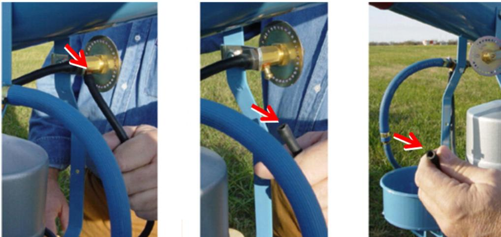
**To prevent accidental detonations, bleed remaining fuel by disconnecting rubber tubing from needle valve.**
