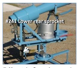
7. Mount the Scare-Away on the Rotomat: Place the Scare-Away on the Rotomat, taking care to fit the chain around the lower rear sprocket (#241).
