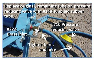
6. Connect Tube under Center Plate: (a) Remove original, remaining tube from yellow pressure reducing valve (#710). **(b)** Connect the pressure reducing valve to the supplied, replacement rubber tube (#148). (c) Connect that tube to the brass inlet (#222) under the center plate. With vice grip or channel lock pliers, tighten pressure rings at this connection, and at connection of the pressure reducing valve.
