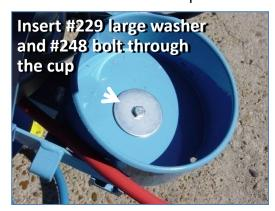
8. Bolt through Cup: Note: Bolt (#248) temporarily holds the bracket (#228) on back of unit. Remove and use for front cup. After chain fits loosely around the two sprockets, and Scare-Away is resting properly on Rotomat, place large washer (#229) over the hole in center of front cup. Screw bolt (#248) into Rotomat brace (#207).
